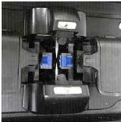
14. Close the electrode cap, electrode replacement is complete
